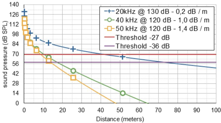
Figure: Approximation of recording distance for two different threshold settings based on typical bat calls. Note the explanations in the next paragraph.
