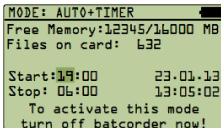
**Start/Stop** controls the automatic start and stop time of the batcorder. Adjust these entries as you like. **Now turn off the batcorder, without switching to another screen** and the Auto+Timer mode is activated.
