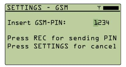
After pushing the **REC** button the PIN is transferred to the SIM-card and the return signal is retrieved. If PIN is correct the GSM-modem tries to dial into the operator's network. If this does not succeed or the PIN is invalid, an error message will be displayed.
