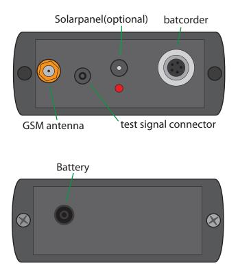
All connections are choosen so each plug only fits exactly in one connector. The battery input is compatible for 6V to 17V batteries. Note that the optional solar panel can only charge 6V batteries. If you are using a 12V battery a 12V panel can be connected as well.
