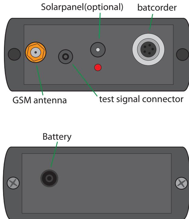
All connections are chosen so each plug only fits exactly in one connector. The battery input is compatible for 6V to 17V batteries. Note that the optional solar panel can only charge 6V batteries. If you are using a 12V battery a 12V panel can be connected as well.
