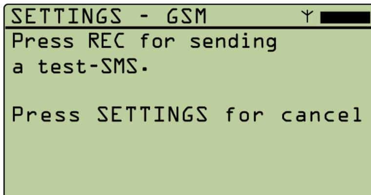
Afterward the batcorder displays whether the test-SMS has been successful or not. If the transmission has been successful and all necessary entries have been made, the batcorder is ready for operating with the box-extension. Both components can then be installed in the nacelle.
