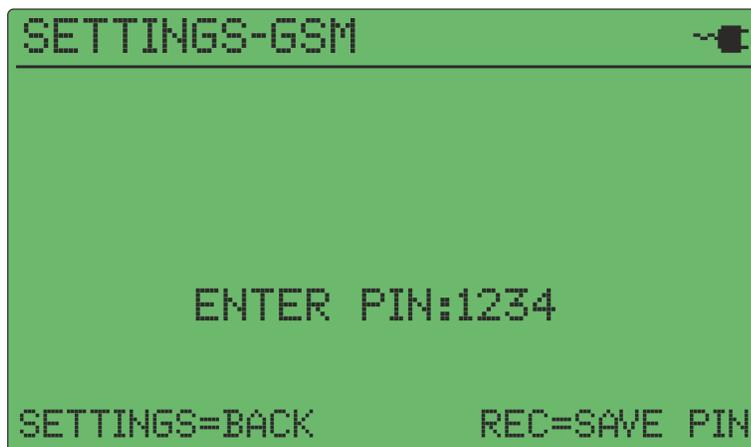
After pressing the REC key, the PIN is transferred to the SIM card and the response is requested. If the PIN is correct, the GSM modem attempts to log into the operator's network. If this does not succeed or if the PIN is invalid, a corresponding error message is output.
