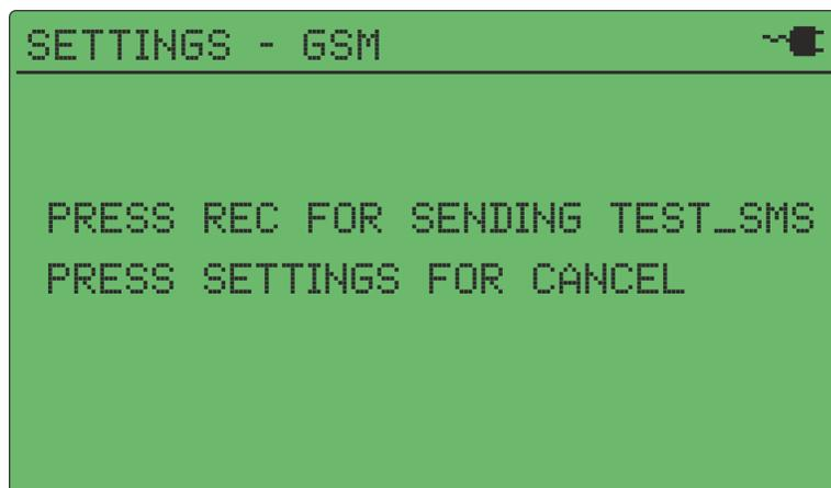
The success of the test SMS will be displayed on the *batcorder* screen afterwards. If the sending was successful and all necessary entries were made, the *batcorder* is ready for operation with the *Extension 4.0*.
