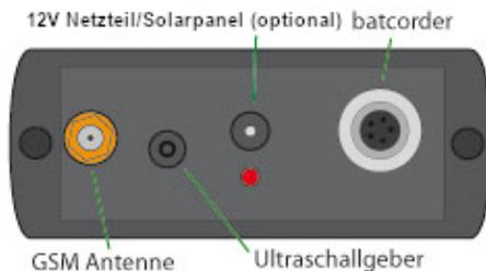
All plugs and sockets are designed so that each plug fits only into the socket intended for it. The battery input is compatible for input voltages from 6V - 17V. Please note that the optional solar panel can only charge 6V batteries.
