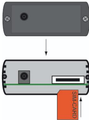
To install the SIM card, open the control module on the side of the battery connection. To open the housing, the two screws (Phillips head) must be removed. Behind them is a circuit board on which the GSM modem is installed. The GSM modem has a slot on the right side, into which the SIM card must be inserted. To do this, carefully push the SIM card into the slot as far as it will go. The contacts of the SIM card must point downwards so that the cut corner is on the front left.
