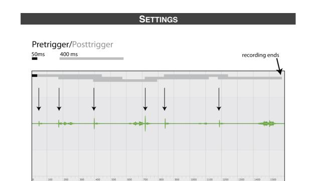
The graph explains pre- and posttrigger times of the *batcorder*. Arrows indicate positive trigger events (= bat calls). The pretrigger of 50 ms is not adjustable.
