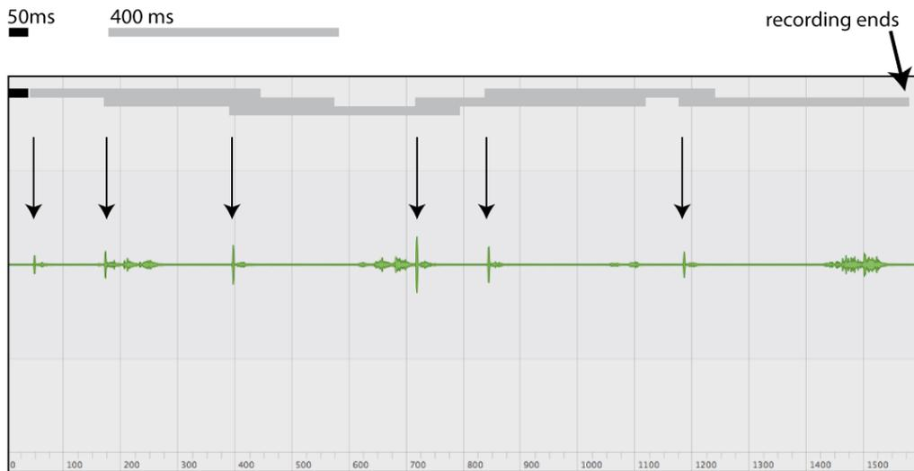
The graph explains pre- and posttrigger times of the *batcorder*. Arrows indicate positive trigger events (= bat calls). The pretrigger of 50 ms is not adjustable.
