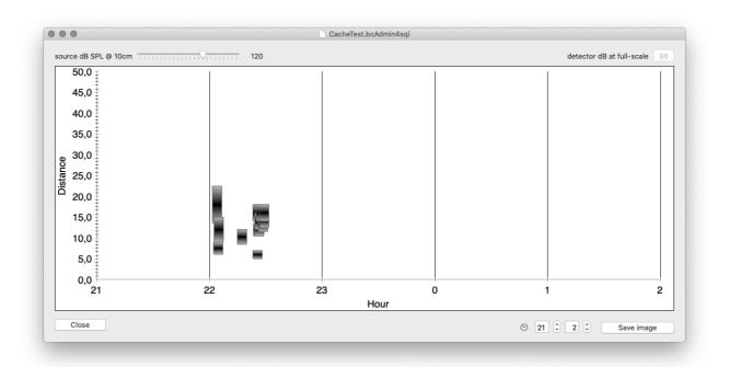
For the batcorder you can assume 96 dB full scale at 40 kHz when properly calibrated. If your detector of another brand is calibrated, you should have a value for full scale as well. Bats can be expected to use sound pressure levels of 90 dB (whispering bats) up to 130 dB SPL.
